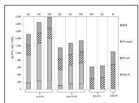
Figure 4 Carbon footprint of different PV systems indicating the solar module carbon emission dominance. Balance of system (BOS) includes typically includes inverters, mounting structures, cable and connectors8
